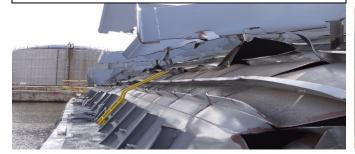
Bulkhead between the #1 from the #2 cargo tank, folded/breached
